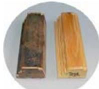
Pine treated with TEKNOL® AQUA 1410 (on the right) and untreated control after accelerated condensation test
