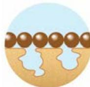
Traditional primers sit on the surface of the timber with limited penetration
